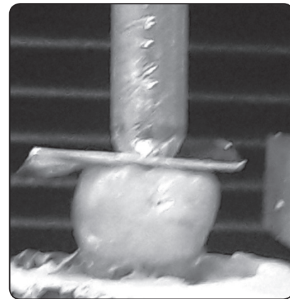
Fig. (4) Axial compressive loading on a tooth specimen in universal testing machine.
