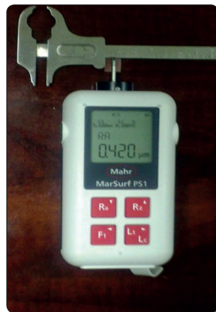
Fig. (1) The pocket profilometer with Stylus pick-up scanning the specimen surface.
