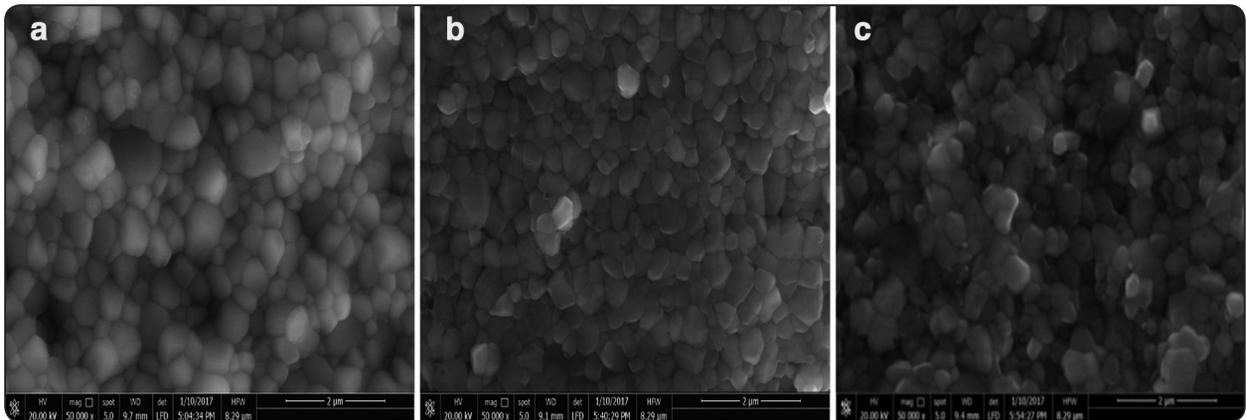
Fig. (6) : SEM images of zirconia samples sintered by A: classic, B: speed and C: super speed cycles without thermodynamic aging and before fracture showing the different grain patterns at 50000x (Top views)
