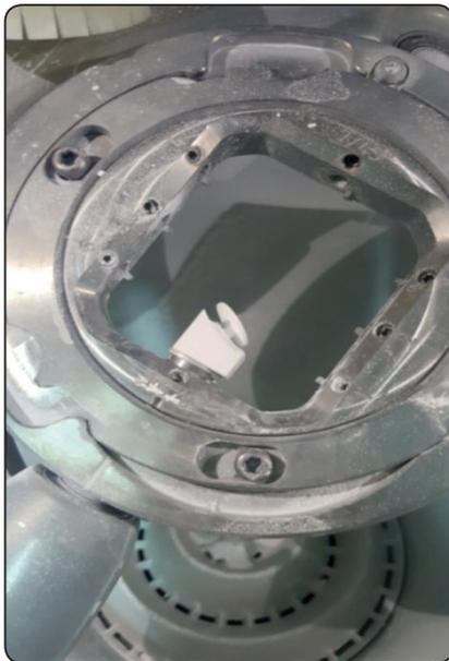
Fig. (1) Milling of the In Coris TZI block in the in Lab MC x 5 milling machine
