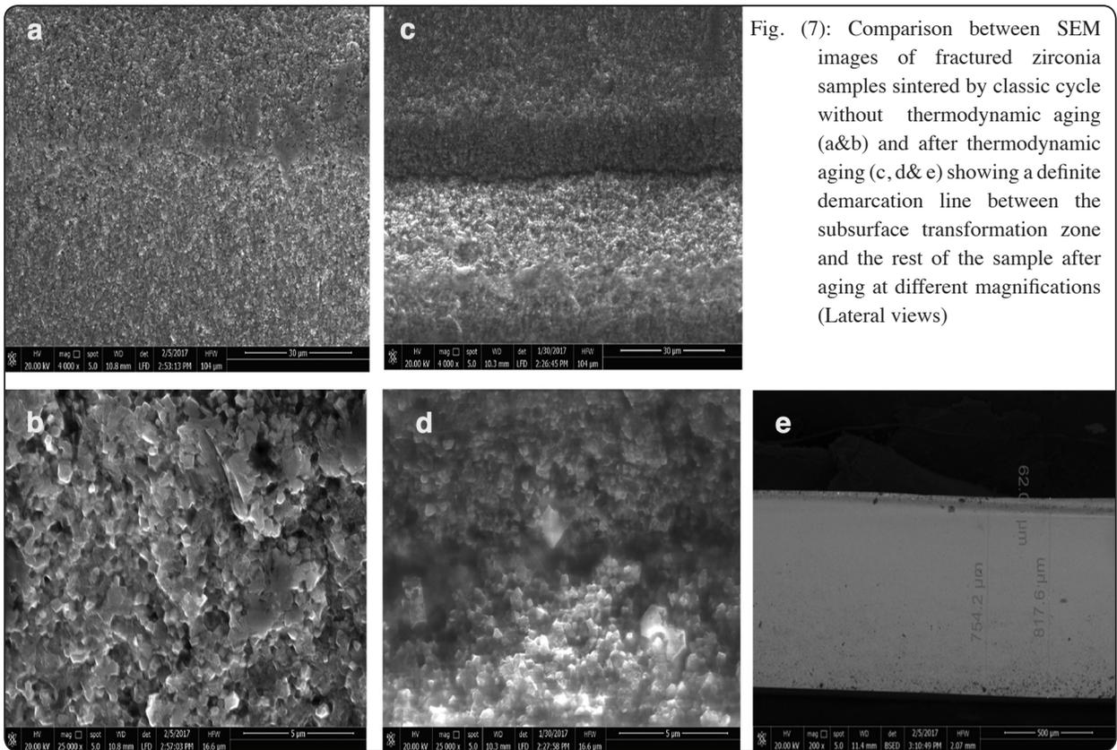
Fig. (7): Comparison between SEM images of fractured zirconia samples sintered by classic cycle without thermodynamic aging (a&b) and after thermodynamic aging (c, d& e) showing a definite demarcation line between the subsurface transformation zone and the rest of the sample after aging at different magnifications (Lateral views)
